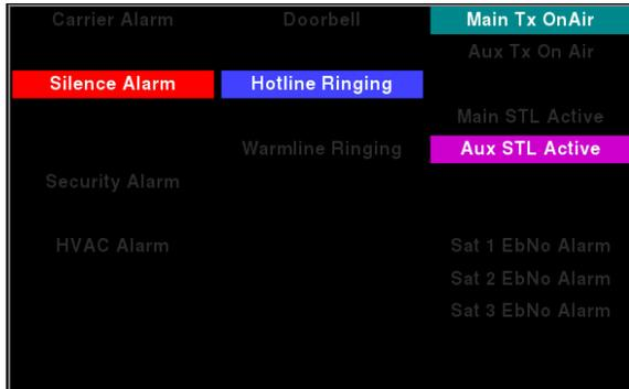
The Notifications Widget is essentially a 'miniature' version of the full-screen display provided by the "Notification Status with Digital Clock" display style, shrunk down to fit within the space provided for a widget. Please see the "Notification Status with Digital Clock" Display Style chapter (below) for information on configuration.
